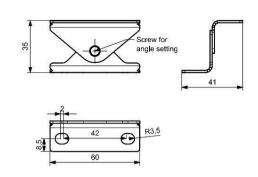
Image with Light Bracket, can also be installed without angle setting bracket.
